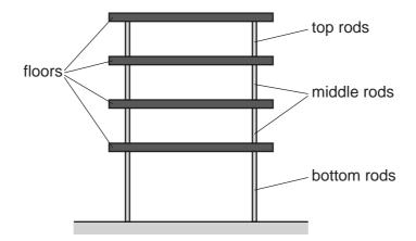
The spacing of the bottom floor from the ground is twice that of the spacing between the floors. Between each floor are equal numbers of vertical steel supporting rods of negligible mass compared with the floors. The rods are of different diameters so that the stress in each rod is the same.
