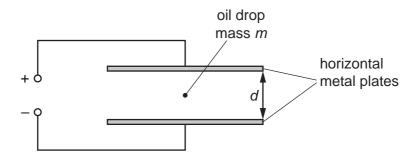
When the potential difference (p.d.) between the plates is  $V_1$  the oil drop rises at a constant speed. When the p.d. is decreased to a value  $V_2$  the oil drop falls at the same constant speed.
