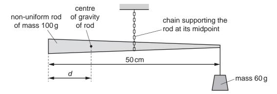
The centre of gravity of the rod is a distance *d* from its left-hand end.
